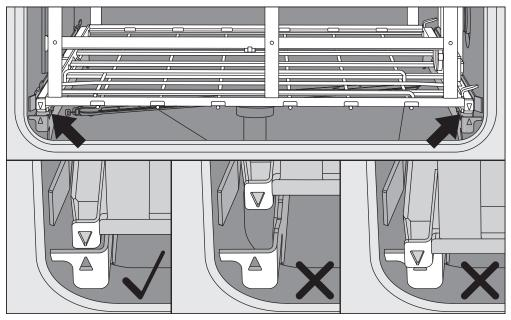
The markings on the load carrier  $\mathbf{\nabla}$  and in the wash cabinet  $\mathbf{\Delta}$  need to be flush with one another.
